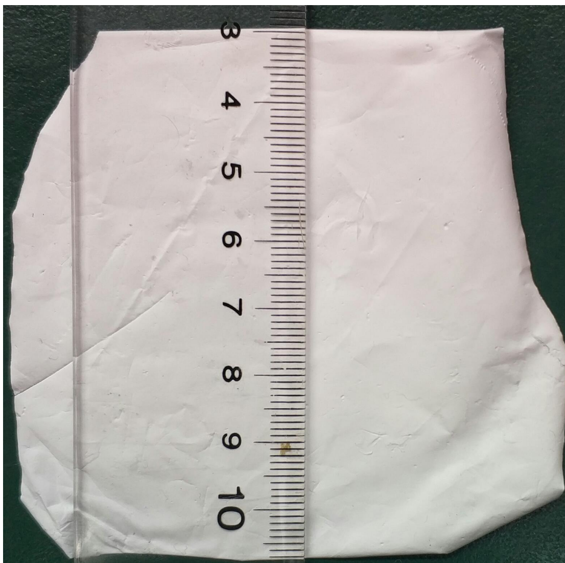
Figure S2. Macroscale image of electrospun nanofibers mat
