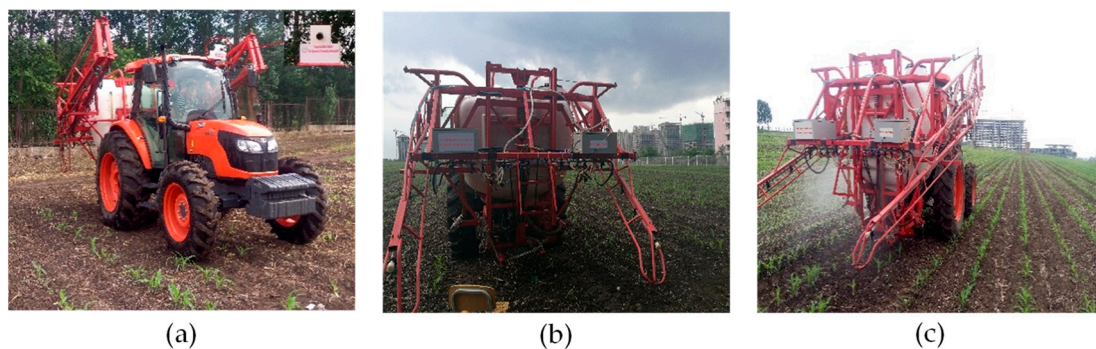
Figure 7. Field validation experiment using the proposed method: (a) Camera placement; (b) Image recognition for target nozzle; (c) Continuous spray.
