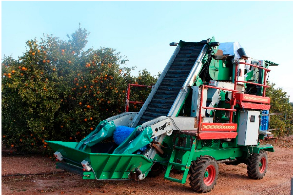
Figure 1. Prototype of a self-propelled harvest-assist platform.
