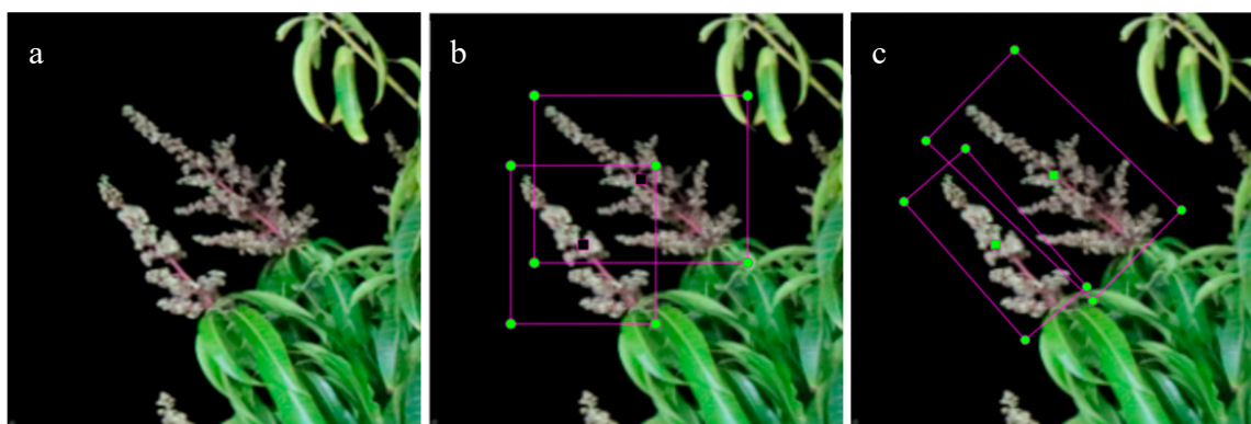
Figure 1. (a) Original image, (b) upright bounding box and (c) rotated bounding box.
