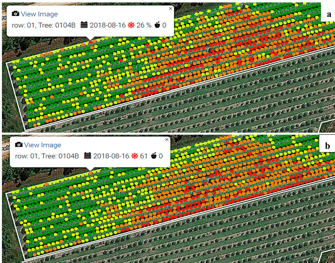
Figure 10. (a) Intensity level and (b) panicle count (using R^2 CNN(-rotated)) of an orchard with tree rows (994 trees, 1988 images). The colours green, orange and red colour corresponds to low, medium and high flowering levels, per tree with each coloured dot representing the image of one side of a tree. In the top panel the categories are in terms of flower pixels as a percentage of canopy pixels (<10%, 10% to 25% and >25%). In the bottom panel, the categories are in terms of total panicle number (<30, 30 to 70 and >70 panicles per tree image).
