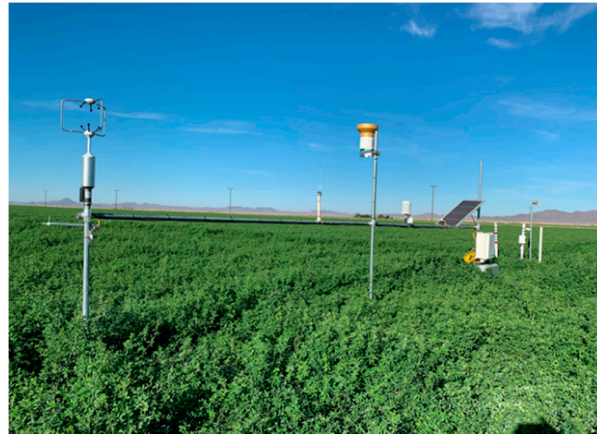
Figure 1. A fully automated surface renewal and eddy covariance evapotranspiration (ET) tower in the plot under normal farmer irrigation practice (NI) at site A3.
