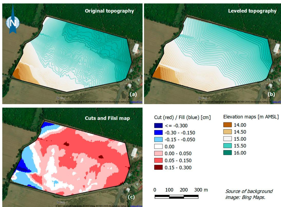
**Figure 4.** 3D surfaces of (a) original topography, (b) VS leveled topography and (c) the respective map of cuts and fills. The contour lines in (b) represent the pattern of the levees that were marked on field after the executing the VS design.
