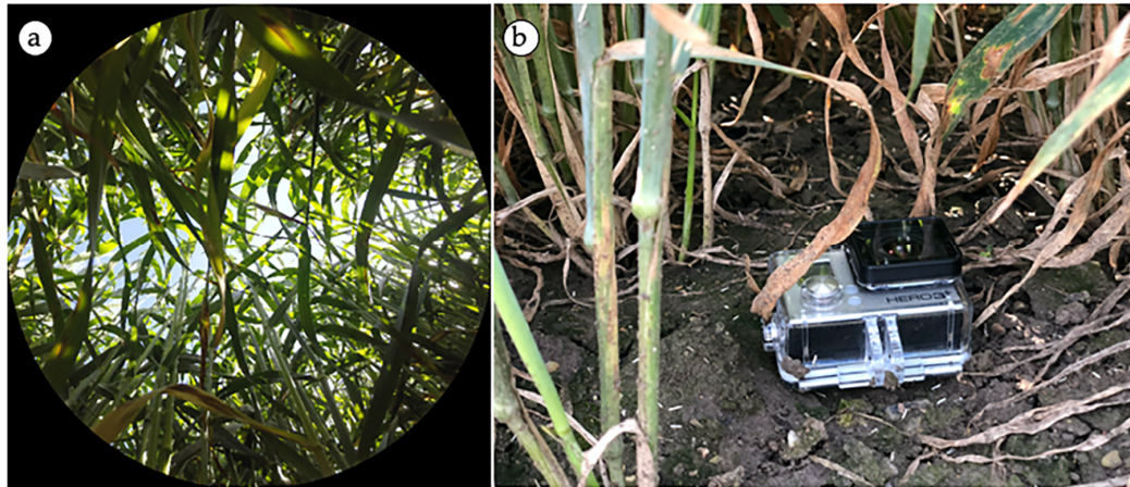
Figure 5. The device (Go Pro camera) used to take the bottom-up hemispherical images during the study (b) and an example of the resulting images (a).
