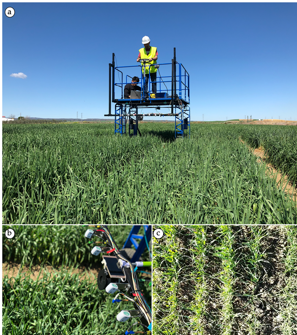
Figure 4. Image acquisition using the high-throughput phenotyping platform (HTPP). (a) A picture of the HTPP platform working in the field. A detail of the way the device was attached to the HTPP and a frame taken with the smartphone are shown in (b) and (c), respectively.
