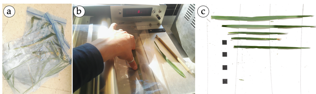
Figure 2. Data collection process for building the allometric relationship. Leaves stored in plastic bags to be transported in a cooler (a); measurements of the unitary leaf area using the LICOR-3100 (b); and leaves placed on a sheet of paper with the squares in the background (c).
