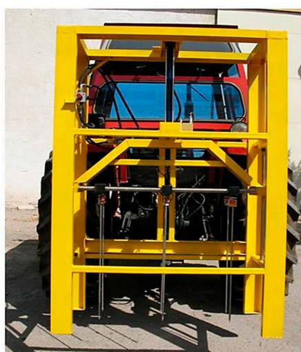
**Figure 4.** Tractor-mounted soil cone penetrometer for measuring the soil cone index.
