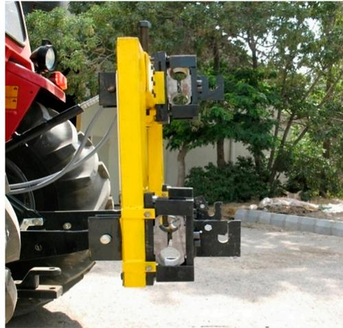
**Figure 1.** Adjustable three-point hitch dynamometer for measuring the draft force of implements.
