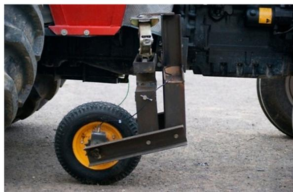
**Figure 2.** Adjustable fifth-wheel to measure the forward speed of the tractor.
