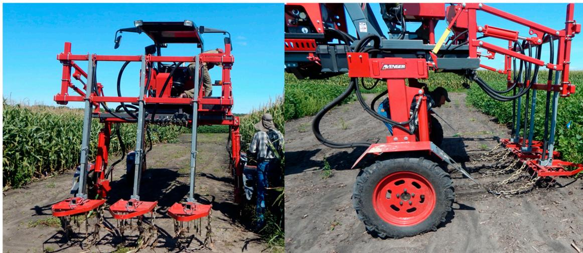
**Figure 1.** Modified Avenger high-clearance tractor outfitted with a Gandy Co. Orbit Air Seeder. Drop stanchions support cover crop seed delivery housing and soil incorporation units. Photo credit: Eric Ristau.
