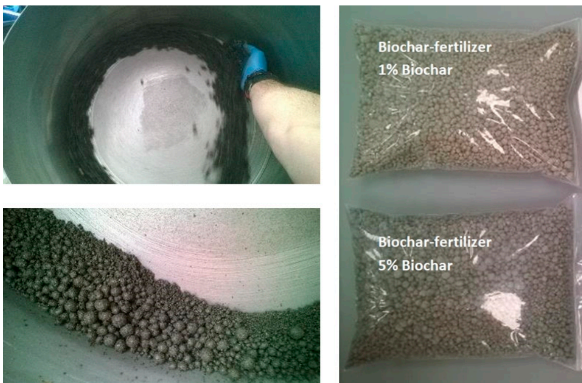
Figure S3: Biochar fertilizer manual manufacturing in rotatory dish.
