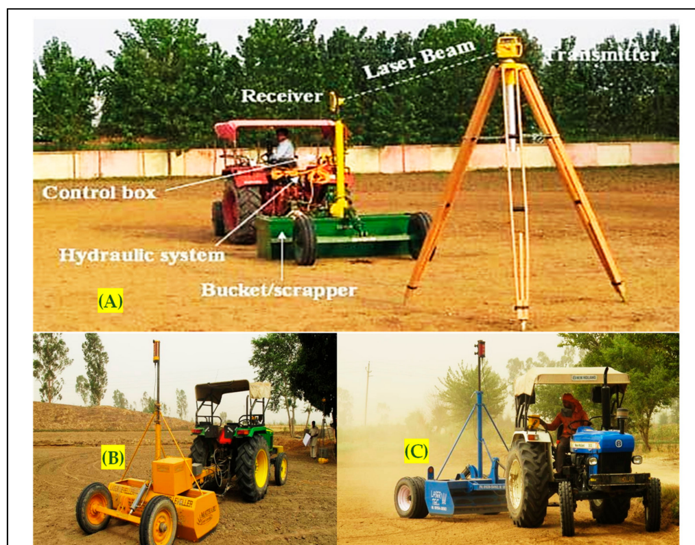
Figure 1. Precision laser land leveling (PLL) in field conditions, (A) showing the function of different components; (B,C) PLL in operation levelling a field.
