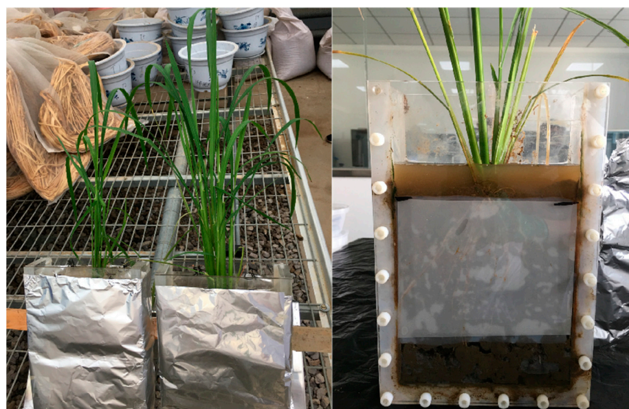
Figure S3. Experimental setup for imaging of the dynamic distributions of multi-elements in rice rhizosphere using LDH s -DGT probe.
