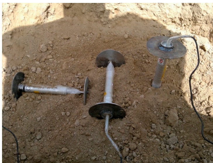
Figure 2. Placement of strain transducers including endplates inside the soil profile in longitudinal, lateral and vertical directions.
