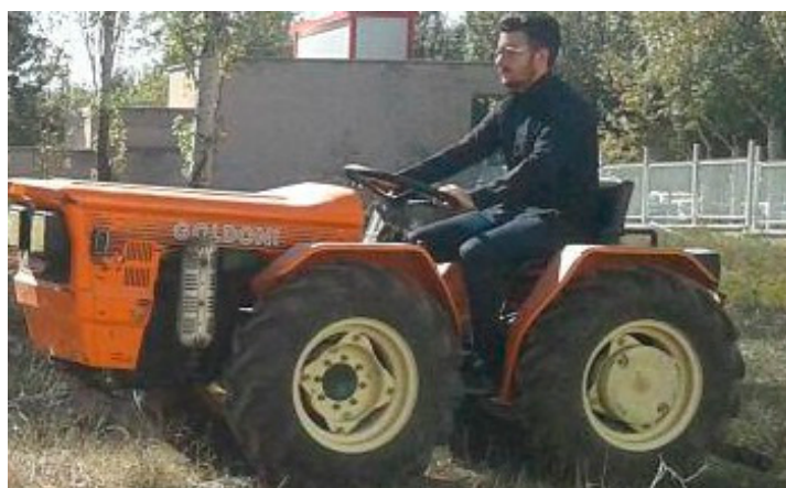
Figure 1. A four wheel drive (4WD) Goldoni model 240 tractor.
