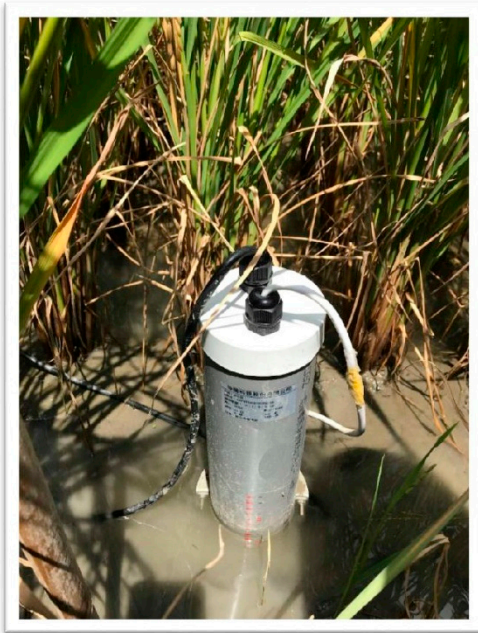
Additional file 1: Figure S1. Intelligent sensor for paddy field. (a) water level sensor (b) remote intelligent water meter.
