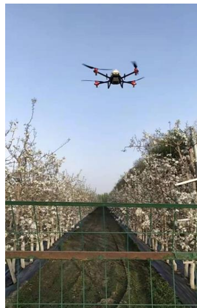
Figure 2. UAV pollination field test.
