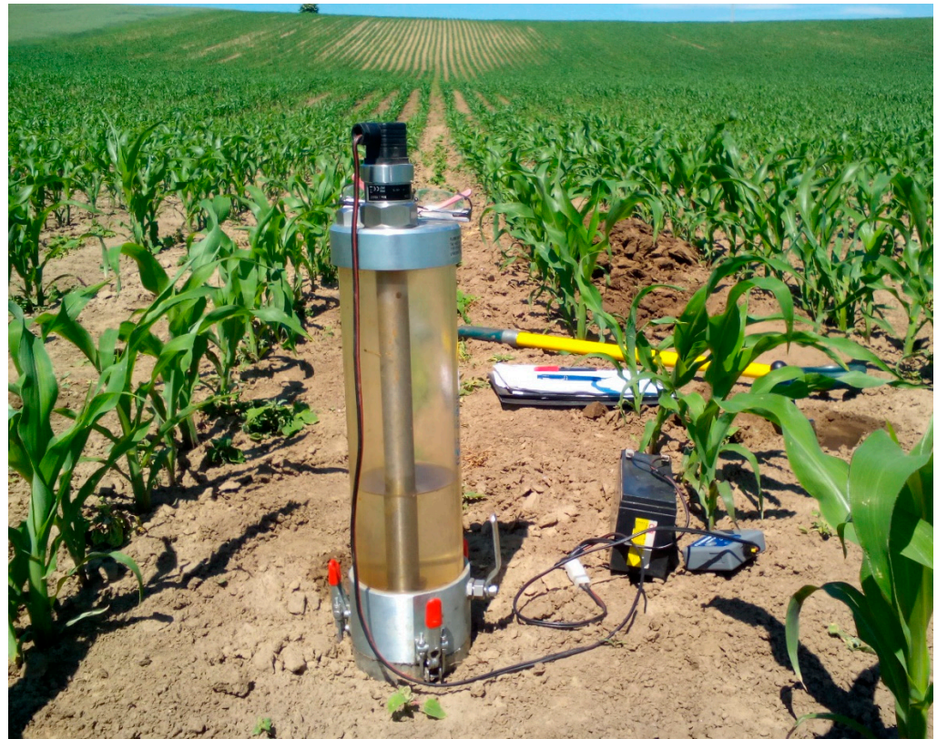
Figure 3. Ponding infiltrometer Flowgroup.
