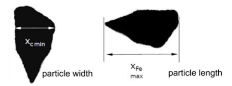
**Figure 1.** Two main particle size parameters analyzed with Particle Analyzer Camsizer: particle width ( $x_{cmin}$ , the shortest chord diameter), particle length ( $x_{Femax}$ , the longest Feret diameter) (adapted from [44].).
