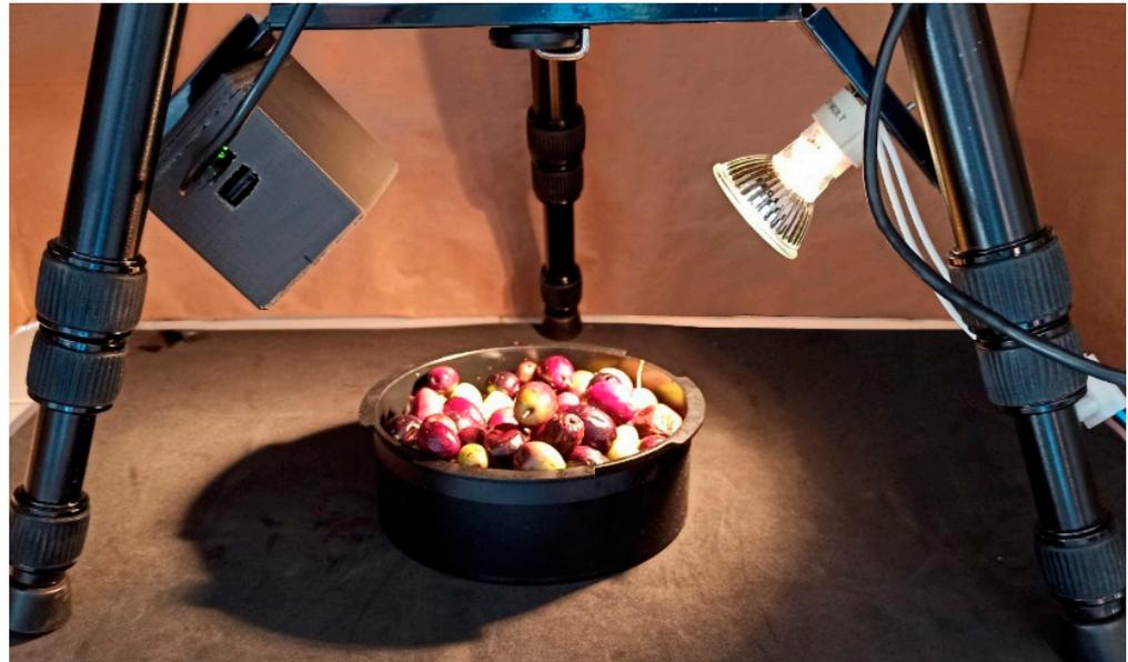
**Figure 2.** Example of an olive sample measurement taken during the spectral data acquisition.
