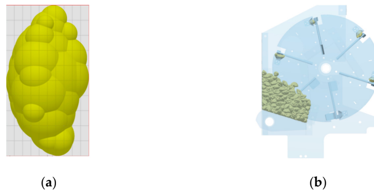
Figure 6. Simulation model and simulation working state diagram. (a) Multi-sphere representation of the garlic seeds; (b) EDEM simulation of the seed rower operating state.
