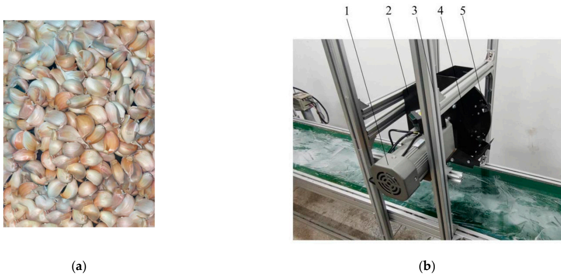
Figure 7. Test materials and bench. (a) Garlic of Pizhou; (b) 1. motor governor; 2. seed-filling chamber; 3. mounting rack; 4. seeding tray; 5. seed-taking device.
