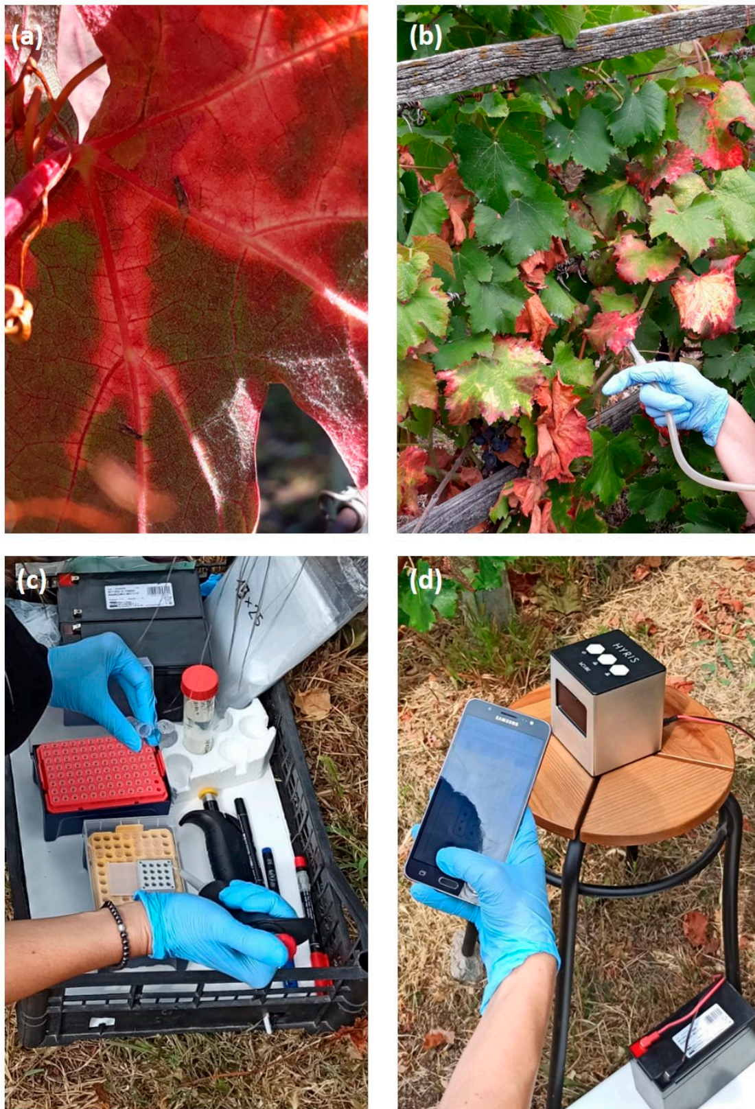
Figure 3. In-field detection of Flavescence dorée phytoplasma (FDp) in Scaphoideus titanus using real-time LAMP assay: (a) adult of S. titanus on infected grapevine leaves; (b) capture of S. titanus ; (c) preparation of insect crude extracts and the LAMP reaction mixture; and (d) set up of the LAMP assay by smart phone and bCube2 instrument running in the vineyard.
