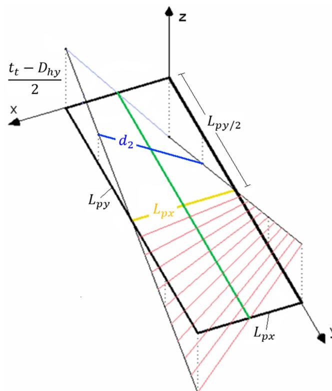
**Figure 5.** Graphic definition of the generatrix  $d_2$ .
