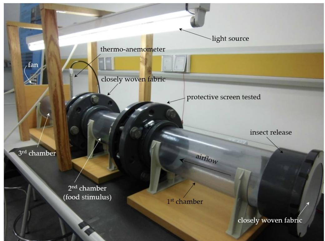
**Figure 6.** Experimental device for measuring the protective efficacy of screens.
