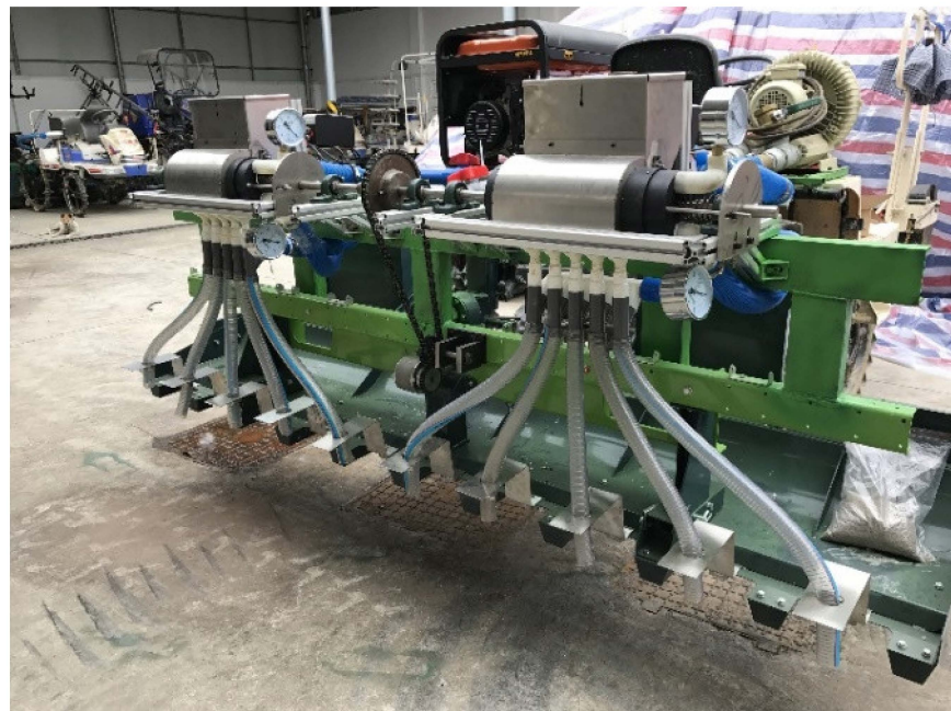
Figure 2. The practicality picture of hill-drop pneumatic central cylinder direct-seeding machine for hybrid rice.
