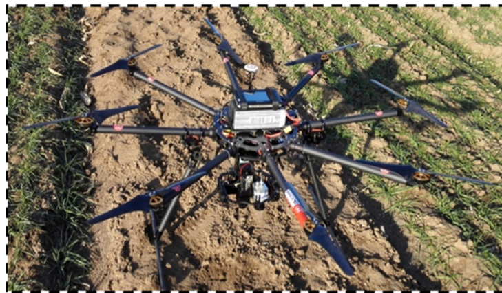
Figure 1. The UAV platform for simultaneously mounting the HD digital and TIR cameras.
