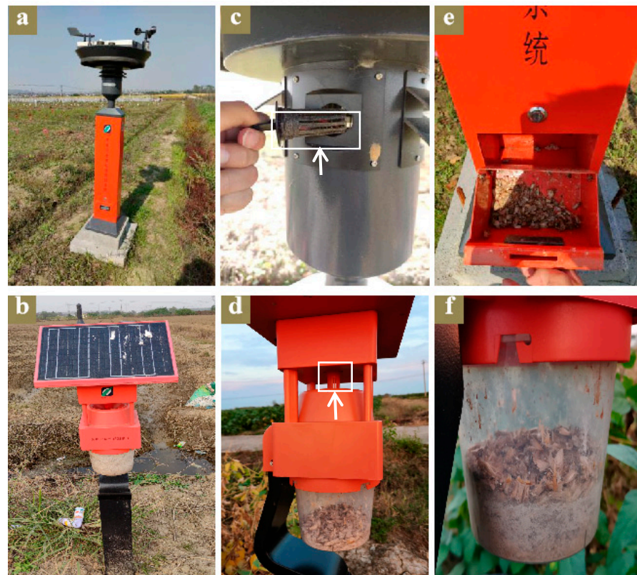
Figure 2. Two kinds of automatic insect monitors, installation positions of pheromone lure and their male collection devices. (a) AIM; (b) AIM-lite-A; (c,d) Installation device and location of pheromone lure (indicated by the white box and arrow in the figure) of AIM and AIM-lite-A, respectively; (e,f) insect collection device of AIM, AIM-lite-A and captured males of S. litura .
