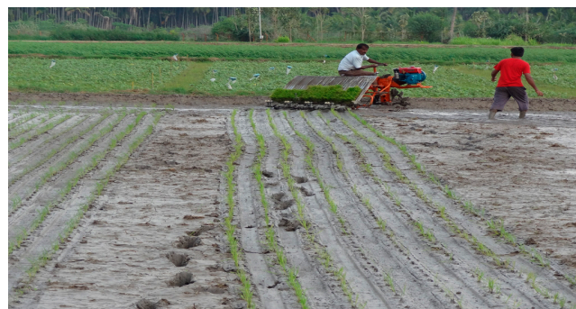
Figure 3. Mechanical transplanter designed at Tamil Nadu Agricultural University for SRI use, transplanting young mat-nursery seedlings, 1–2 hill ^{-1} with a spacing of 23 \times 23 cm that permits mechanical weeding of the field in perpendicular directions.
