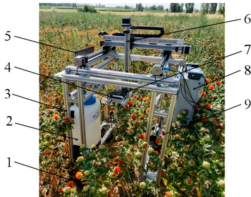
Figure 1. The overall structure of the safflower-picking robot. 1. Walking device; 2. collecting box; 3. machine frame; 4. visual recognition system; 5. calculator; 6. three-axis linear slide; 7. end-effector; 8. electronic control box; 9. mobile power.
