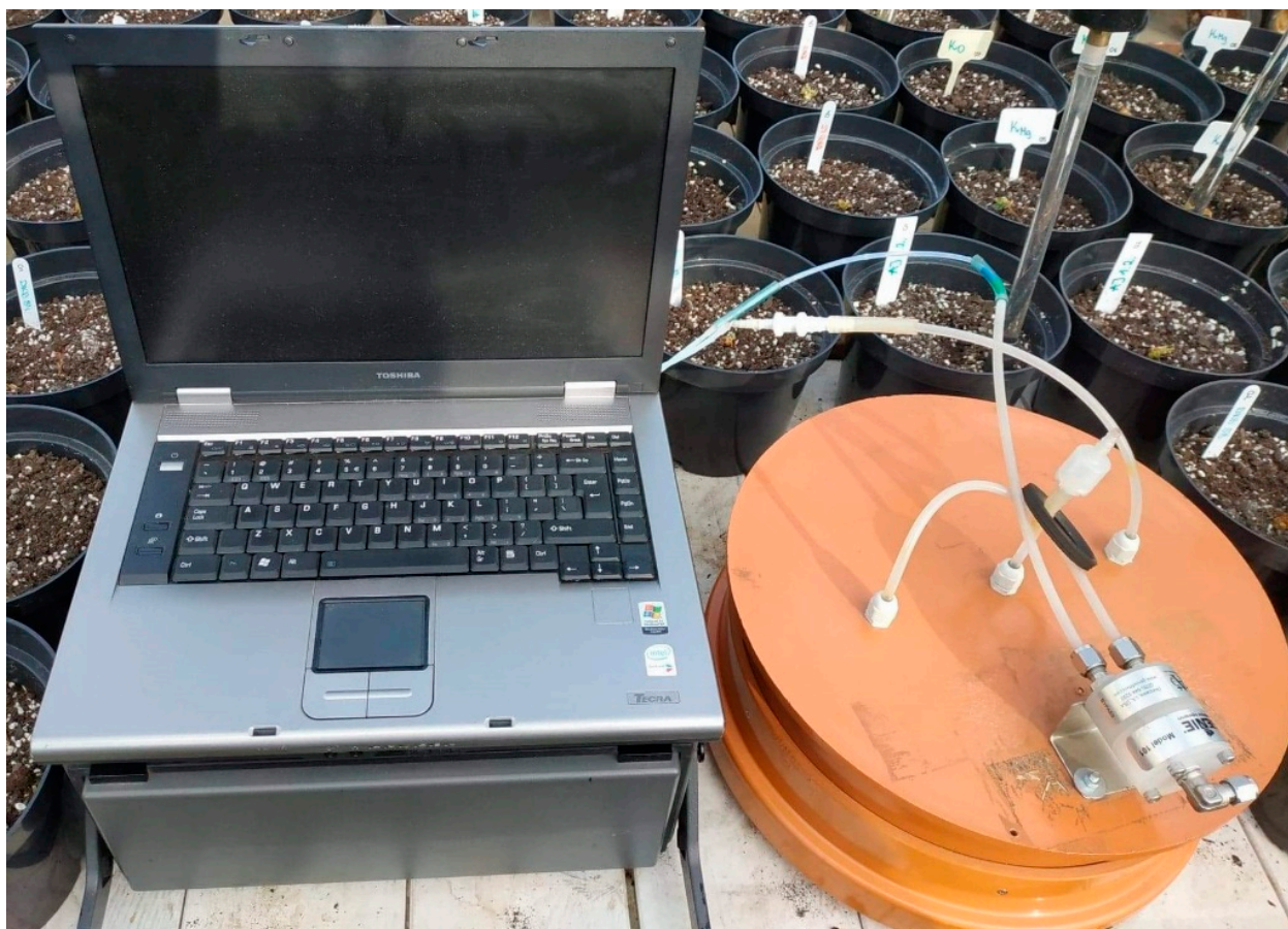
Figure 1. Photoacoustic gas meter 1412 INNOVA Air Tech Instruments with a static chamber for measuring gas emissions and immissions.
