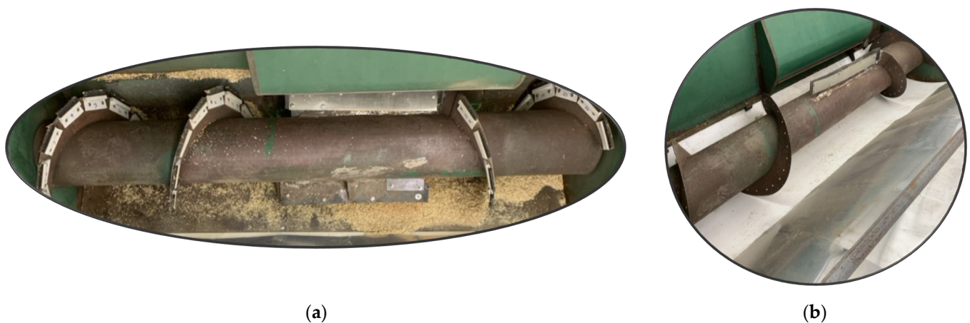
Figure 4. Auger redesign implementation: (a) brush concept and (b) shim concept.
