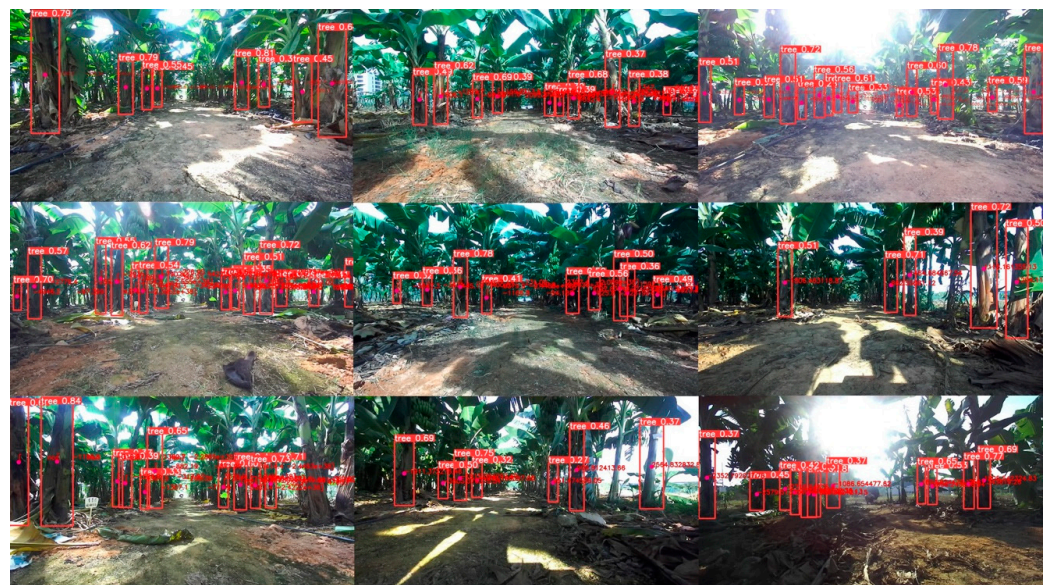
Figure 14. Examples of trunk detection in a banana orchard. Red boxes represent the detected trunks and the numbers above the boxes represent the detected confidence.
