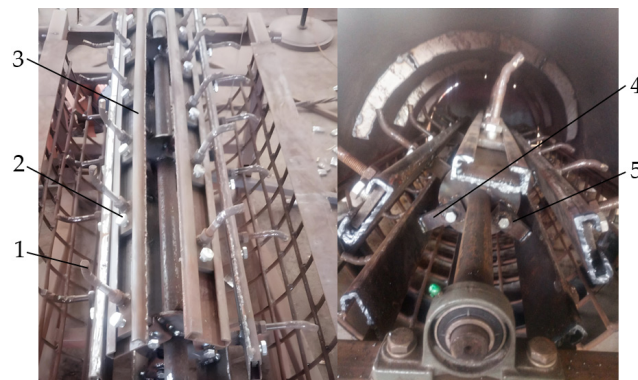
Figure 3. The internal structure of the pod-picking roller: 1—bending tooth; 2—axial slider; 3—axial sliding chute; 4—radial slider; 5—radial sleeve.
