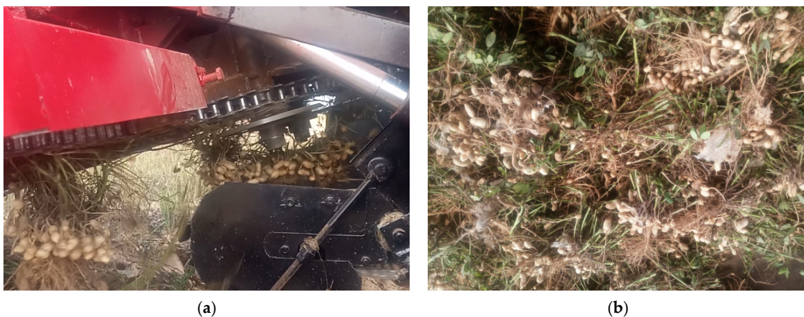
Figure 8. Acquisition of peanut root disk. (a) The front-end double disc cutter of the combine harvester separates the peanut root disk from the peanut plant. (b) Peanut root disk.
