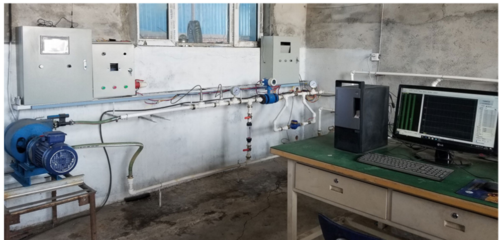
Figure 10. Flow regulation test platform.
