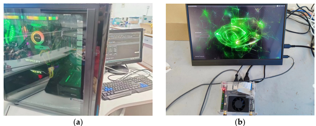
Figure 9. Experimental device. (a) Experimental device utilized for training the model; (b) Jetson TX2.
