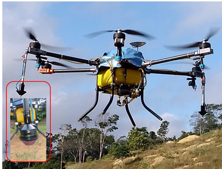
Figure 1. Multirotor unmanned aerial vehicle (UAV) and centrifugal nozzle used in the spraying experiment.
