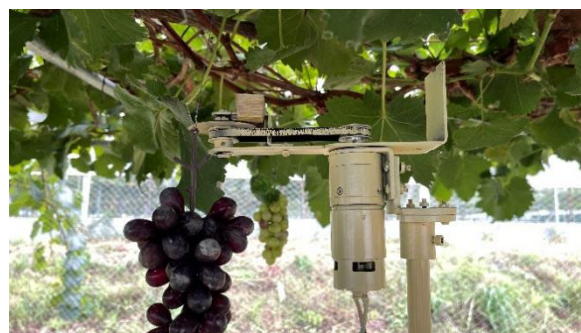
Figure 23. Relative position between the end of the end effector and the picking point of the fruit.
