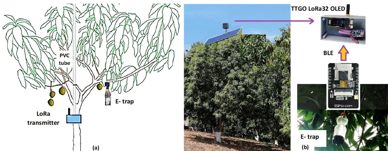
Figure 5. (a) Schematic diagram from a tree having the LoRa module at the trunk. (b) Main modules were used to take images at the trap and send signals from the top of the tower.
