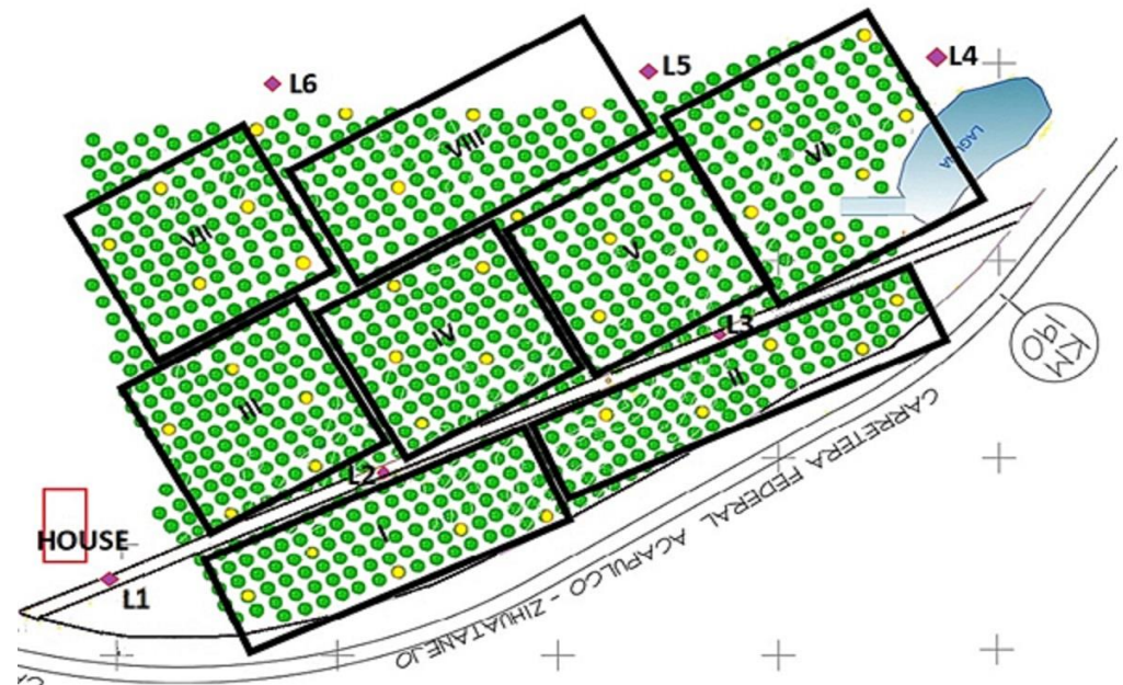
Figure 1. E-traps and transmission sites in the 8-hectare mango orchard. Green circles represent mango trees, and yellow circles show trees with e-traps. Violet diamonds represent transmission towers.
