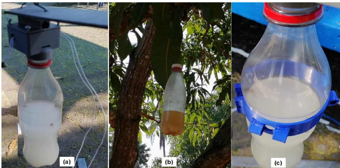
Figure 14. (a) PET trap hanging in the lab. (b) PET trap hanging in the tree after 3 weeks with the same bait. (c) PET trap surrounded by a plastic structure to avoid movement.
