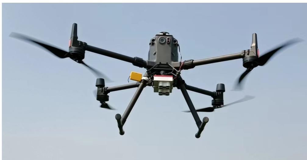
**Figure 2.** Matrice 300 RTK UAV and RedEdge multi-spectral camera.
