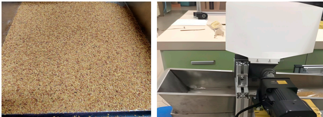
Figure 9. The uniformity test of the plasma seed treatment device. Left: The uniformity test process. Right: The vibration-uniform material distribution device.
