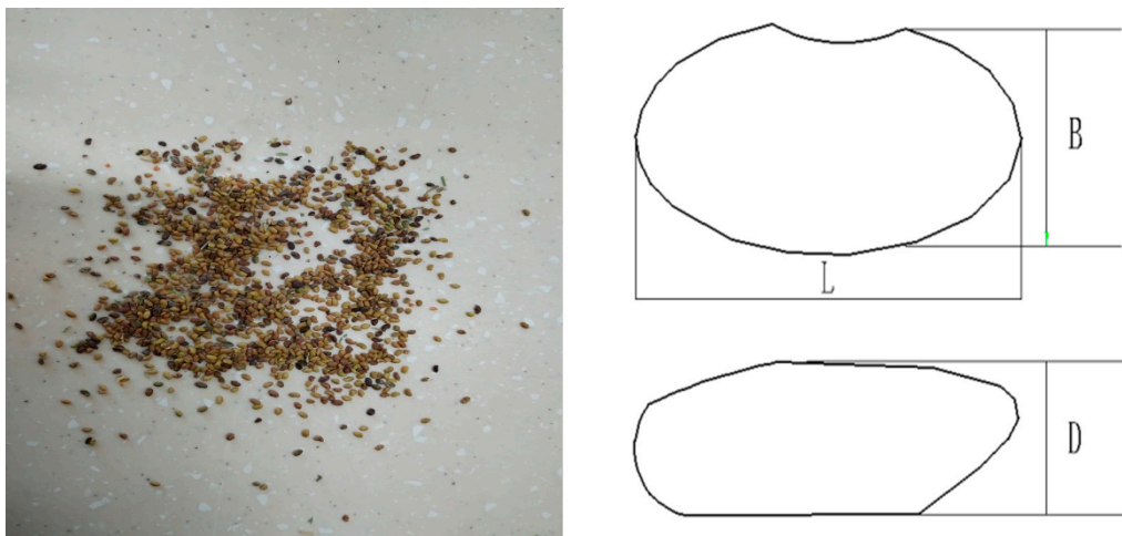
Figure 1. Alfalfa seeds. (Left): Alfalfa seeds physical picture. (Right): Alfalfa seed size diagram (“L” means “long”, “B” means wide, and “D” means “high”).
