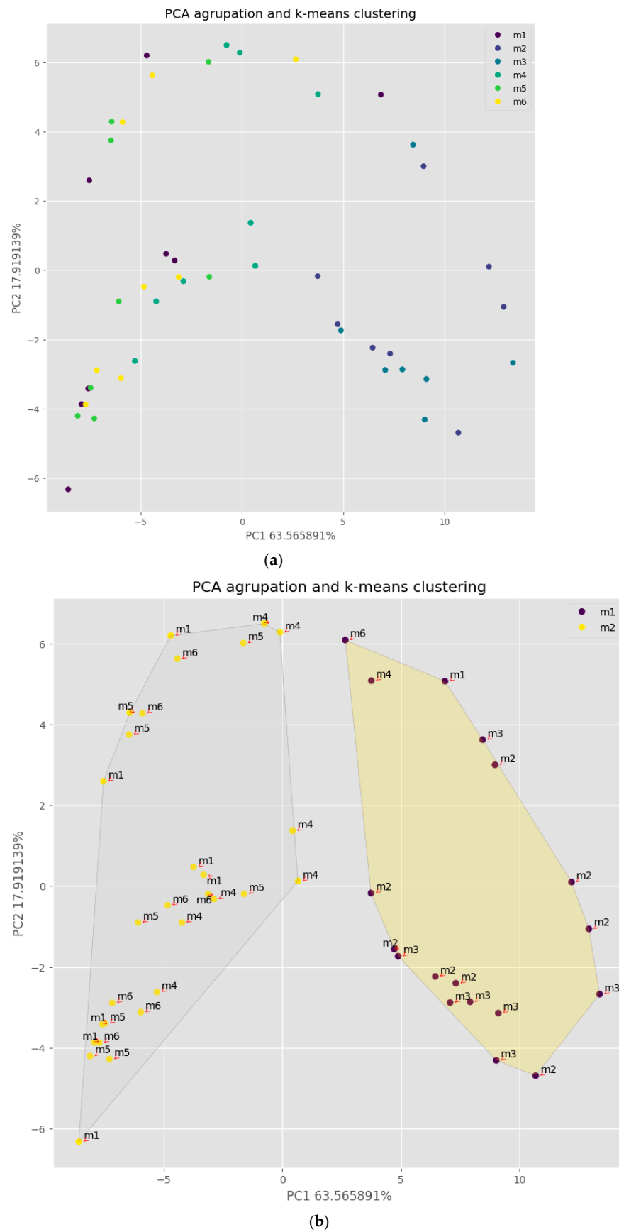
Figure 6. Results of the PCA analyses in the preliminary study: (a) Graph showing the PCA analysis of all the samples and each color indicates to which of the 6 types of samples each point belongs. (m1,
