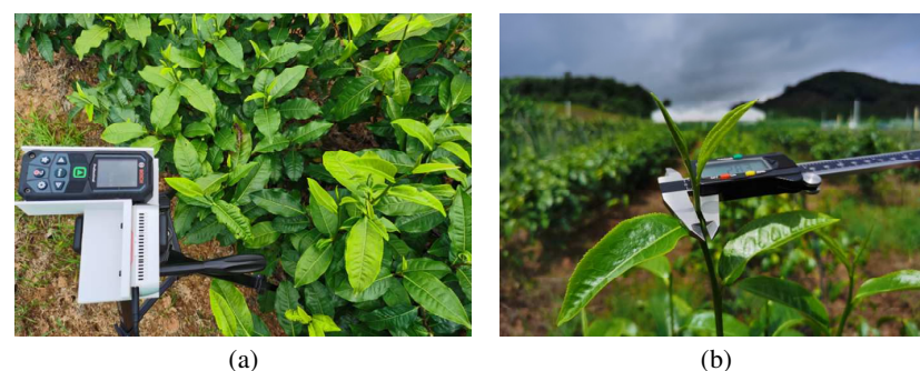
Figure 10. Schematic diagram of the measurement. (a) Distance measurement, (b) Diameter measurement.
