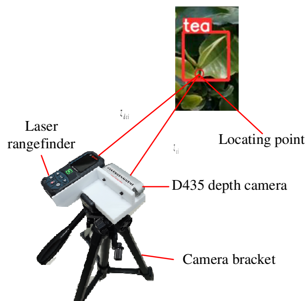
Figure 8. Graph of distance measurement.
