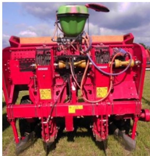
Figure 2. Planter with mounted dressing device; source: own.
