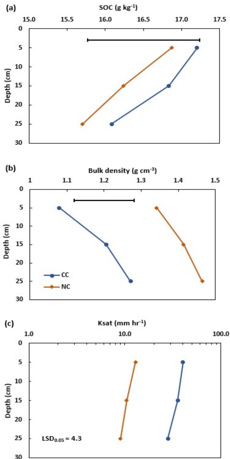
**Figure 2.** Soil properties relative to depth during the study period: (a) soil organic carbon (SOC), (b) soil bulk density, and (c) saturated hydraulic conductivity ( $K_{\text{sat}}$ ). Bar represents LSD at 0.05. Due to log scale, the LSD value for  $K_{\text{sat}}$  is provided rather than using a bar for the representation. Note: CC = cover crops, NC = no cover crop.
