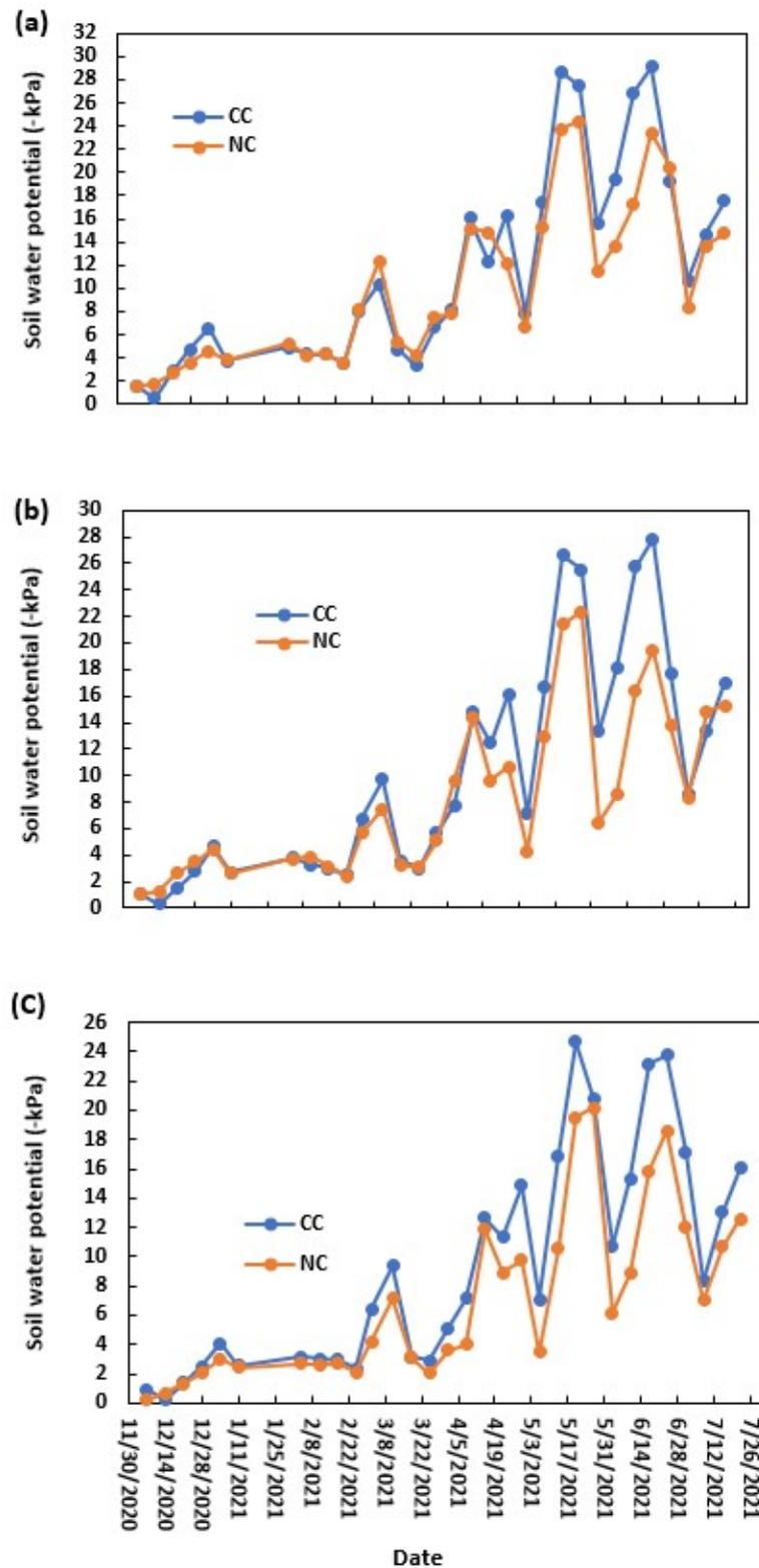
Figure 3. In situ-measured soil water potential at (a) 5 cm, (b) 15 cm, and (c) 25 cm at the research site. All dates are in the MM/DD/YYYY format.
