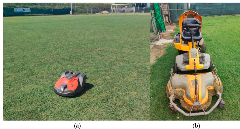
Figure 2. The two different cutting systems in the selected soccer pitch: (a) the autonomous mower with systematic trajectories and (b) the ride-on mower.
