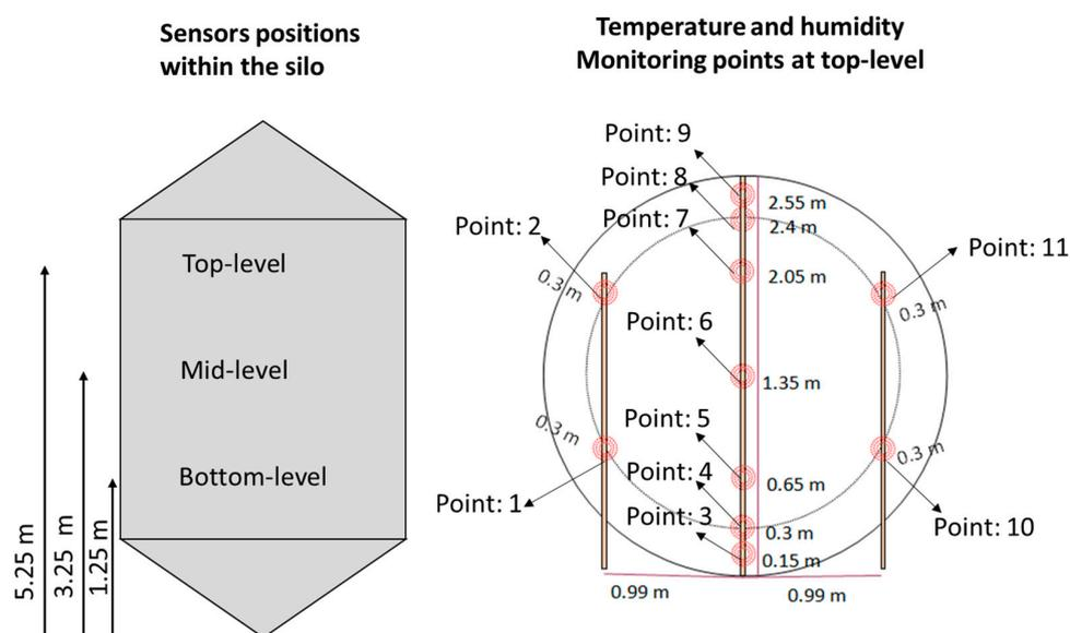
**Figure 5.** Schematic diagram illustrating the positions of sensors at different heights within the silo and subsequent eleven monitoring points of temperature and humidity at the top level (5.25 m from the base). The same number of monitoring points were applied at the same positions at the mid- (3.25 m from the base) and bottom levels (1.25 m from the base).
