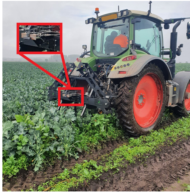
Figure 2. The data capture process using cameras mounted to the rear of a tractor. The position of the camera is highlighted with a red box.
