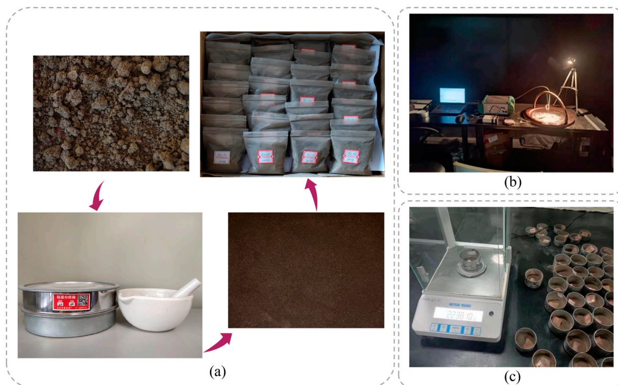
Figure 2. Soil sample processing flow. (a) Dried soil samples are ground, filtered, and divided into two portions. (b) Soil spectral data collection. (c) Soil moisture determination.
