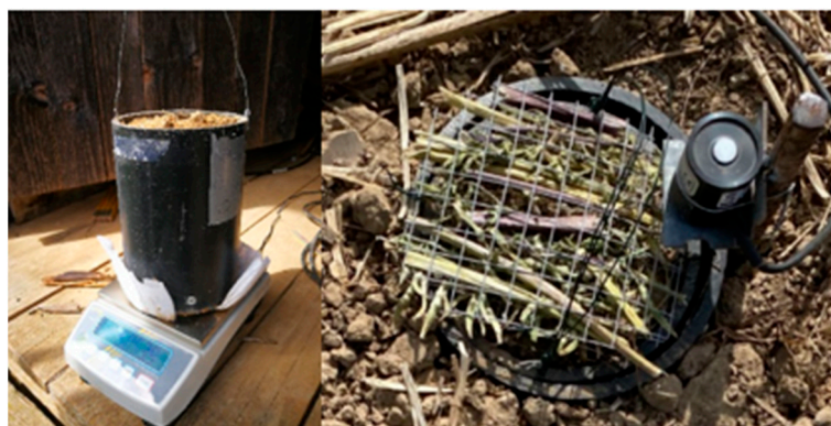
Figure 4. Weighing process of mini-lysimeter without mulch (left); pyranometer and litterbag added to mini-lysimeter (right).
