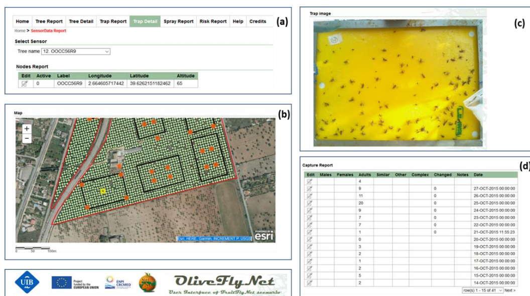
Figure 7. Output of the OliveFlyNet application interface showing details about the real-time insect counting system (ReTIC) system based on analysis of pictures sent by the e-traps. (a) Node report, (b) Node location, (c) Trap image, and (d) Capture report.
