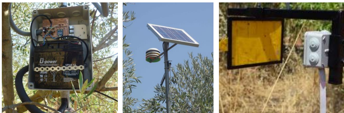
Figure 4. Electronic components of the e-trap. Left: Battery and electronics. Center: Upper part of the e-trap showing solar panel and Stevenson screens that protected temperature and relative humidity (HR) sensors. Right: Camera placed in front of a Rimi ® trap.
