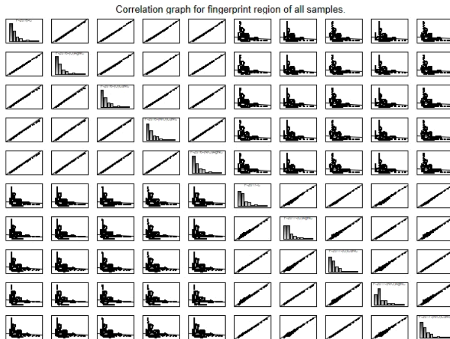
Figure 4. Plot of the pairwise correlations between the oil samples from the FT-IR spectra. Diagonal values are measures of sampling adequacy for individual fingerprint regions of oil samples; off-diagonal are anti-image correlations. In the case of high values of correlation, we have (nearly) linear dependence, otherwise nonlinear.
