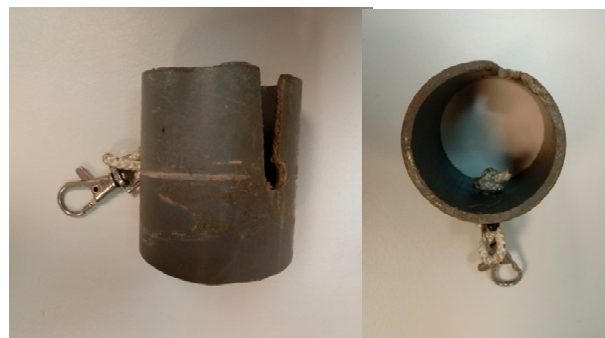
Figure 3. The gripper device used for green fruits.
