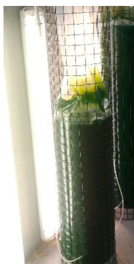
Figure 1. Vertical-column photobioreactor used for the production of microalgae.
